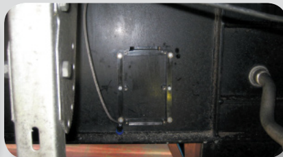
Mounting bracket is bolted to the trailer
