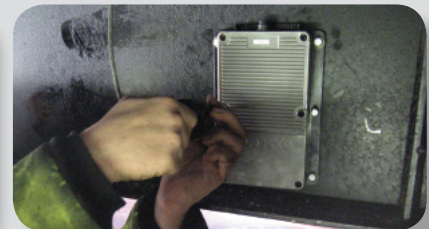
DCU screws into the mounting bracket
